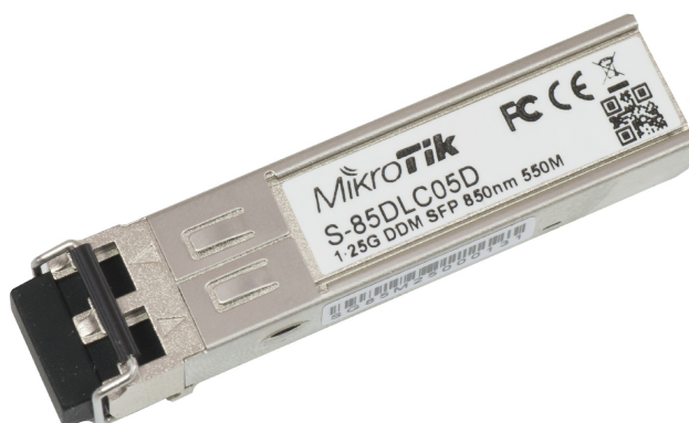
Figure 7.11: Fiber Optic SFP Module
